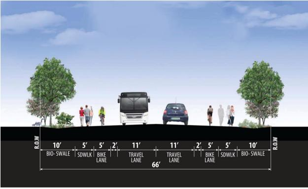
PROPOSED CROSS SECTION OF N. PALAFOX ST. IMRPOVEMENTS, CREDIT: ATKINS GLOBAL N. PALAFOX CORRIDOR MANAGEMENT PLAN, 2015
